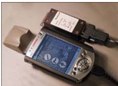
Fig. 7: The PDA with the compass and GPS attached
